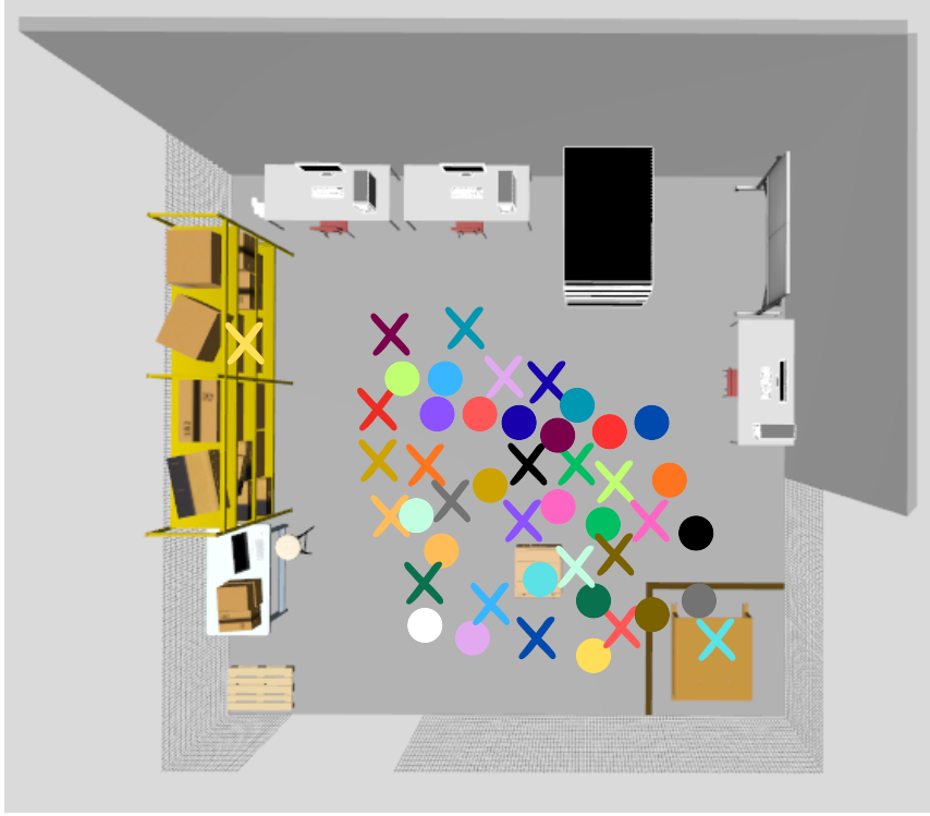
Figure 13: Different initial testing positions of the trolley and the robot in simulation environment 1, where × represents the trolley location and • represents the robot location.
