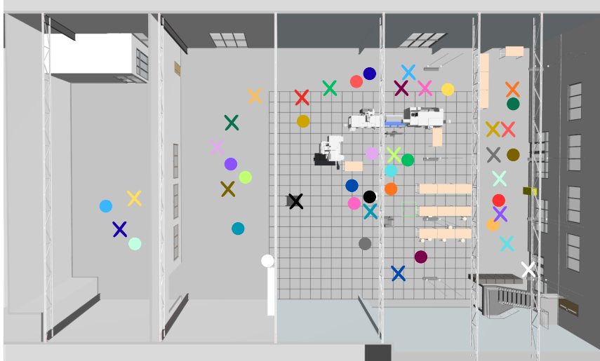
Figure 15: Different initial testing positions of the trolley and the robot in simulation environment 3, where \times represents the trolley location and \bullet represents the robot location.
